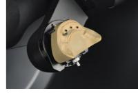
The special scanning strategy for long-span, implant level screwretained suprastructures determines implant positions with high precision
